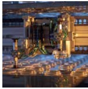
Vacuum operated suction cup picks block-pieces
